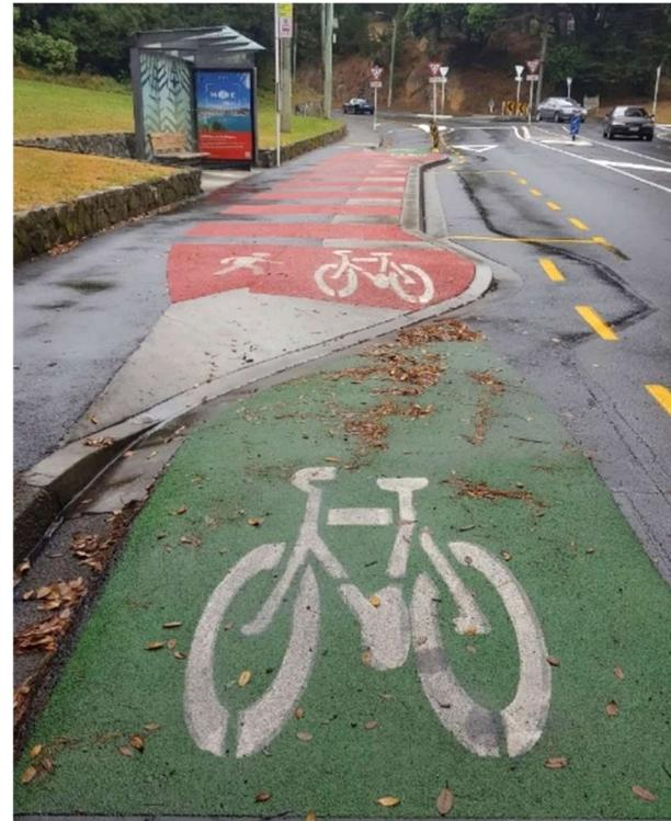
Cycle lane transitions onto footpath and passes between bus shelter and bus bay. Shared zone for cyclists and pedestrians is denoted by red stripes and painted symbols. Site is on an uphill gradient.
